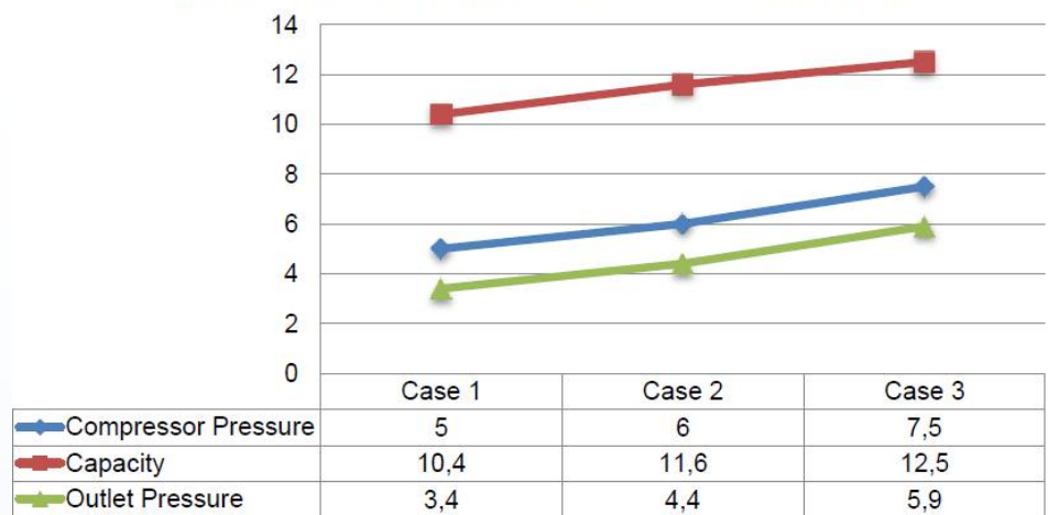
Oxygen Generator Compressor Pressure - Output Capacity - Output Pressure Graph
